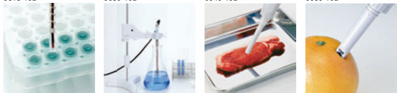
Precious, trace amount sample Direct measurement from micro tubes, only 50µL of sample required For large containers and long test tubes 283 mm length & 8 mm diameter Surface of solid samples Gel-like materials such as agar medium, foods such as meat, cloth and paper surface Inside solid samples Measurement inside the solid sample such as fruits, vegetables and bread
