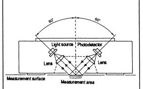
Gloss as measured by the IG-320 is a numerical value which expresses the intensity of the luminous reflection on the surface of an object. The value is determined by comparing the value obtained with a standard reflective surface to the intensity of reflected light on the measurement object.
