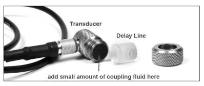
When measuring, press against the top of the transducer with the thumb or index finger to hold the transducer in place. Moderate pressure is sufficient, as it is only necessary to keep the transducer stationary, and the delay line seated flat against the surface of the material being measured.
