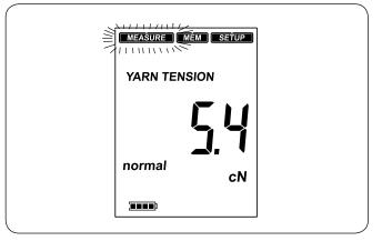
► The yarn tension is shown in "cN" on the display.
