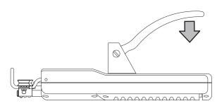
Piece alone. (This is especially true with models rated 20 Kg and higher.) Adding the Lever Assembly shown here will greatly reduce the effort required to open and close the 3-roller system. The Lever Assembly must be installed by the factory or an authorized service facility.
