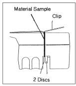
instruments (1000 grams and higher) are usually furnished with a Thickness Compensator, as shown here. To determine whether the Compensator needs to be used for a specific application, take readings with and without the process sample in the Compensator using a hanging weight approximately equal to the process operating tension.
