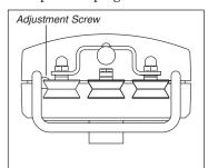
pointer swings. The amount of damping is set by turning the small slotted screw or hex-head screw of the damping assembly located near the guide-roller mounting bracket. The Air Dashpot must be installed at time of original manufacture. It cannot be added later.
