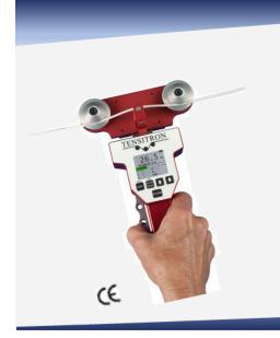
Reliable tension testing for medium-sized wire and other materials
