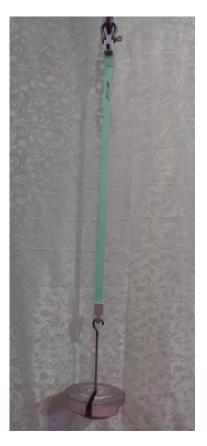
Figure 7: Free hanging weight simulating band tension.
