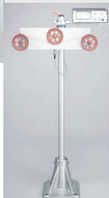
Special solution for measurement of optical fibres roller diameter 100 mm 480 mm measurement path
