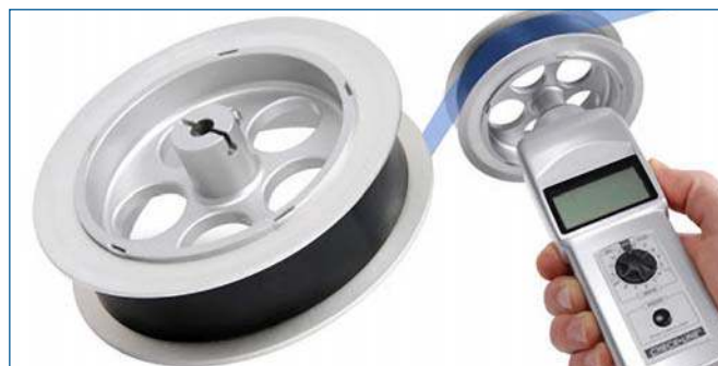
Optional 12" Wheel for Large Diameter Cables, Tapes & Bands.
