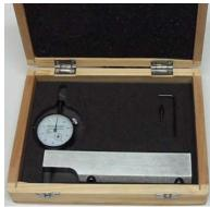
The Reaching + Pit Gauge offers the equipment inspector many advantages over our Basic Pit Gauges (N88-2 or N88-3), with its Dial Indicator mounted at the end of the 152mm (6") Blade, fitted with a long Cut-Away Nose.
