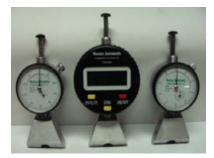
Like all of Western Instruments Dial Pit Gauges, and as illustrated to the left, Pocket Pit Gauges are available in 3 models; Metric, Imperial, and Digital. Western supplies, Pocket Pit Gauges as a Kit, and include; Wood Case, Pocket Pit Gauge Blade, Dial Indicator (Metric, Imperial, or Digital), Allan Key, extra Contact Point, Manual, and Calibration Certificate. They also make a great addition to a custom Kit!
