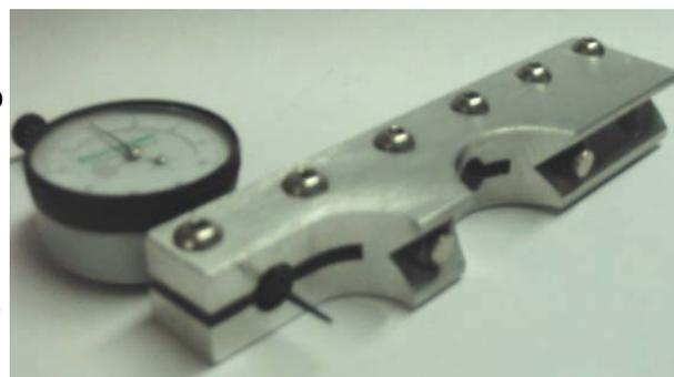
The main benefit of the Reference Gauge® is it tends to be Self Aligning on a round workpiece. When Assembled in the Bridging version, with Connector and End Blades, it is obvious when the Inverted 'V' Edge is not aligned. Like all of our Dial Indicator Pit Gauges, the Reference Gauge® is available as a Metric, Imperial, or Digital model.
