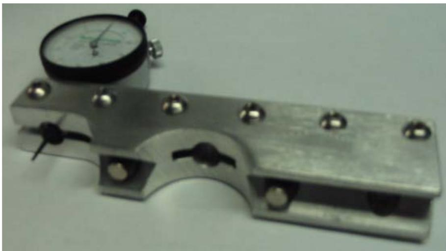
The Reference Gauge®, as illustrated to the left is also fitted with our exclusive Magnetic Hold Down Cartridges, identical to those used on our Standard Magnetic Pit Gauges.
