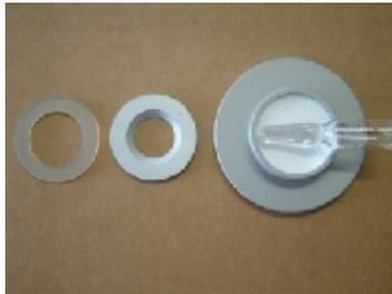
Put in the first gasket ring in the upper part of the calibration device. Push in the Sensor-sword in the upper part as shown at the picture. Now put the second gasket ring into the upper part.
