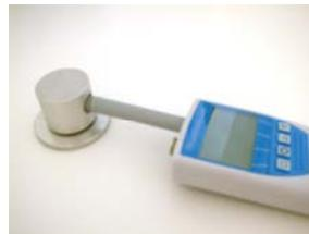
Take the upper part with the RHx and attach these carefully at the bottom part of the calibration device. Screw it up like shown in the picture
