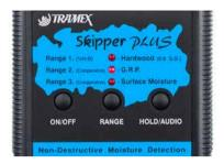
Press Skipper Plus fully against the surface of the material
