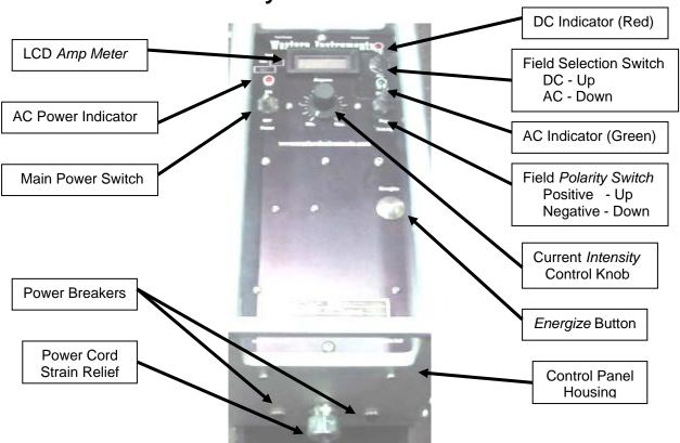
Note: These Operating Instructions also apply to Separate Power Supplies provided as retrofits to other manufacturers Coil Assemblies. Western Instruments makes no claims or warranties when used with other manufactures Coils.
