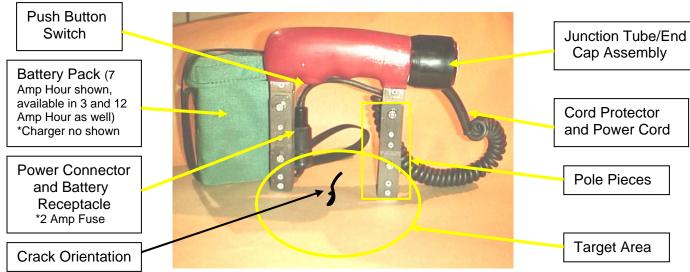
Solid State Push Button Switch – The Solid State Push Button Switch was designed for comfort and safety. While depressed, the switch delivers power (12 Volts DC) to the coil encapsulated in the Yoke housing.
