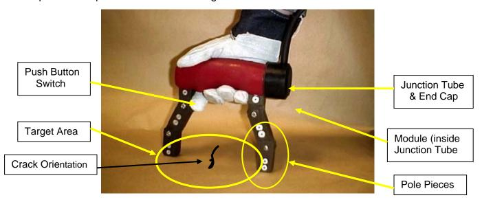
Solid State Push Button Switch – The Solid State Push Button Switch was designed for comfort and safety. While depressed, the switch delivers power (AC) to the coil encapsulated in the Yoke housing.
