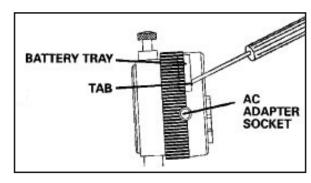
2. Insert two batteries, "+" side up, into tray cavities, then slide the tray into its bezel slot, taking care that the batteries stay in proper position.
