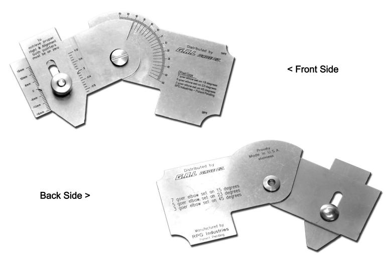
The Offset Gauge can be used to measure the offset between two plates over welds, fit-up bars, landing rings or any other object up to and including 1" that might obstruct quick measuring of two plates where the Bridgecam Gauge might fail.
