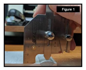
Measuring the Leg of the Fillet Weld (Figure 2)
