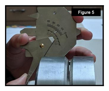
Measuring the undercut of a weld (Figure 6)
