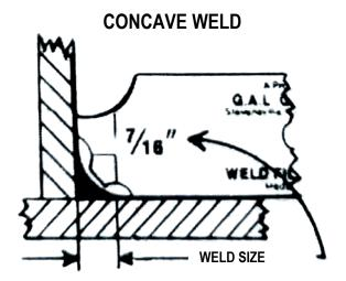
Place double arc edge flush to the base material so tip touches vertical member. If the tip between the double arc touches the center of the weld, the weld is the profile desired and is the size indicated.
