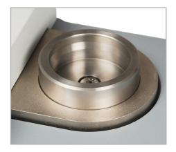
WT3003 Machinable blank terminal fixture For unique sample shapes and sizes.
