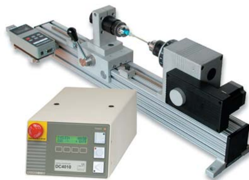
The TSTMH-DC is shown in a pen cap torque test, with a Series STJ torque sensor, BGI force/torque indicator, and G1022 Jacobs chuck grip
