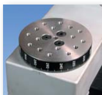
Rotating torque plate has a matrix of tapped holes for grip or fixture mounting
