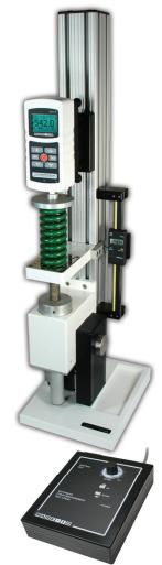
The TSFM500 is shown in a typical spring testing application, with Model M5-1000 digital force gauge and compression plate.
