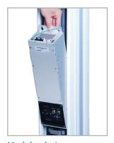
Modular design Most electronics are housed in an integrated enclosure, easily accessible and removable for updating and service.
