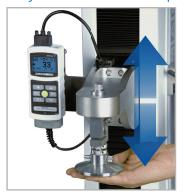
FollowMe™ dynamic positioning Using your hand as your guide, push and pull on the load cell or force gauge to move the crosshead. Responsive enough for quick positioning as well as fine adjustments.
