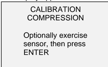
Optionally exercise the load cell shaft several times (at full scale, if possible), then press **ENTER**.
