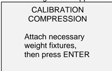
Attach weight fixtures (brackets, hooks, etc), as required. Do not yet attach any weights or apply any calibration loads. Press **ENTER**.
