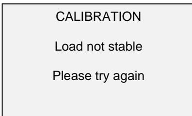
Ensure that the load is not swinging, oscillating, or vibrating in any manner. Then try again.
