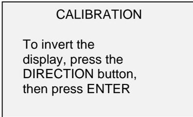
Reverse the orientation of the load cell shaft by rotating the gauge 180 degrees. Press **DIRECTION** to invert the display. Then attach weight fixtures. The following screens will step through the same procedure as with the compression direction. Proceed in the same manner.
