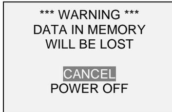
If no option is selected, this screen will be displayed indefinitely, or until battery power has been depleted.
