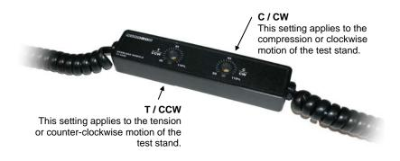
Once the percentages have been set, set up the test sample and proceed with the motorized test. When the force or torque threshold has been reached, the stand will stop moving, the module will produce a constant audible tone and the indicator below the potentiometer will be lit. The tone and indicator light will not turn off until the force or torque decreases to below the threshold value.
