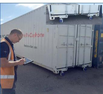
Plot the distances between your load cells in the grid template in the software.
