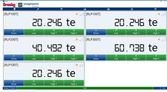
An example of INSIGHT in actual use lifting a refinery installation weighing >500T using a custom made lifting truss and 12x 100T Radiolink plus.
