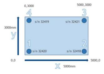
Now you will get read-outs of the load placed on each load cell, total weight, as well as a display of the center of gravity. The larger the circle the larger the weight.
