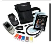
**Comes complete** with PosiTector gage body, FNS probe, precision plastic shim(s), protective rubber holster with belt clip, wrist strap, 3 AAA alkaline batteries, instructions, protective lens shield, convenient carrying case, Long Form Certificate of Calibration traceable to NIST or PTB, USB cable, PosiSoft Software, two (2) year warranty.
