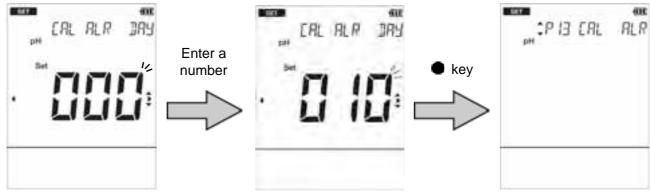
To return to the measurement mode, press the \( \cdot \) key.
