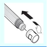
6 Shake the electrode to remove any air bubbles remaining on the ion selective membrane.
