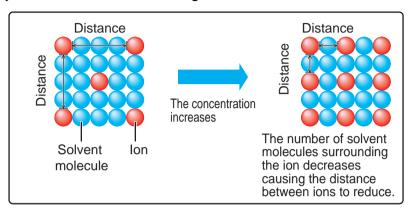
Fig. 7 Difference in state of solution depending on ion concentration
