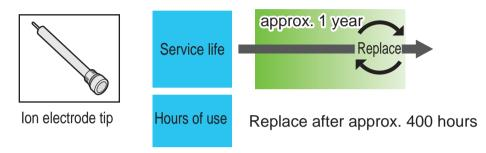
Replace consumables at the period whichever occurs first; approx. one year after purchase or after approx. 400 hours of use, depending on sample solution, measurement frequency, and measurement environment.
