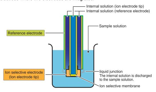
Fig. 4 Structure of combination type ion selective electrode
