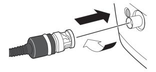
When disconnecting the electrode from the meter, disconnect it in the opposite direction from step 1.
