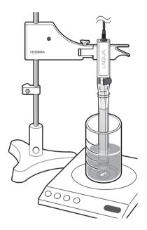
• Do not touch the stir bar with the electrode. It may damage the electrode.
