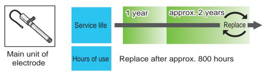
Replace consumables at the period whichever occurs first; approx. two years after purchase or after approx. 800 hours of use, depending on sample solution, measurement frequency, and measurement environment
