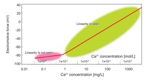
Fig. 8 Calibration curve of calcium ion selective electrode
