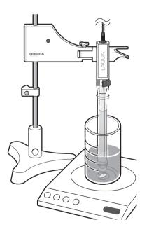
Do not touch the stir bar with the electrode. It may damage the electrode.
