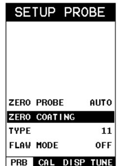
8. Press the **OK** key to zero the coating and return to the **PRB** menu, or **ESC** to cancel the coating zero process.
