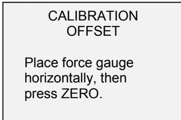
5. Place the force gauge horizontally on a level surface free from vibration, then press **ZERO**. The gauge will calculate internal offsets, and the display appears as follows:
