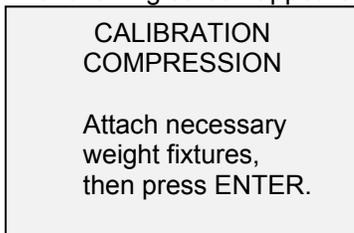
Attach weight fixtures (brackets, hooks, etc), as required. Do not yet attach any weights or apply any calibration loads. Press **ENTER**.
