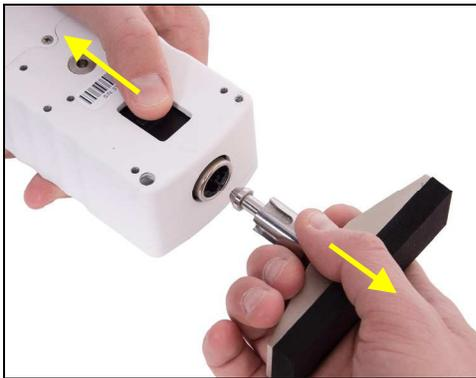
If the E1011 grip adapter (pictured below) is used, common grips and attachments may be mounted via the integrated 5/16-18F thread.
