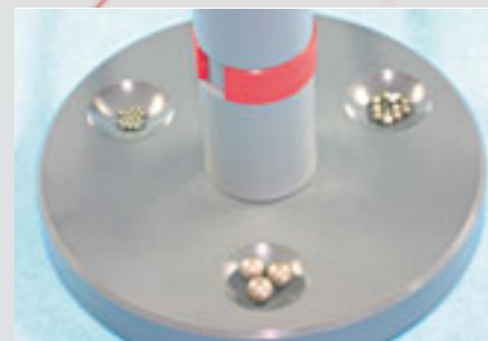
Sensor stand with grooves to hold steel balls in place
