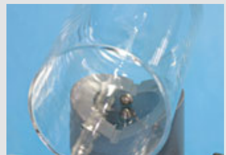
Reference balls with a specially coated finish and dimensional precision to obtain maximum reproducibility of readings.
