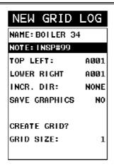
1) Use the arrow keys to scroll through the setup options until **NOTE** is highlighted.
