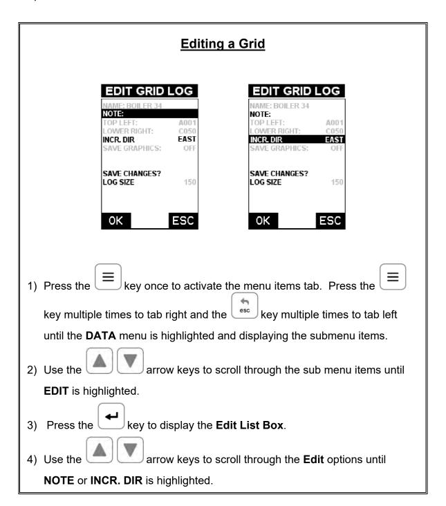
Note: If editing the INCR. DIR, simply use the arrow keys to scroll NONE, NORTH, EAST, SOUTH, WEST for a Grid, or INC, DEC for a Seq Log. Proceed to step 10.
