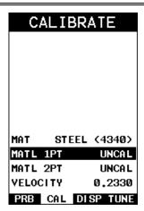
**Note:** Be sure a probe zero has been performed prior to calibration.
