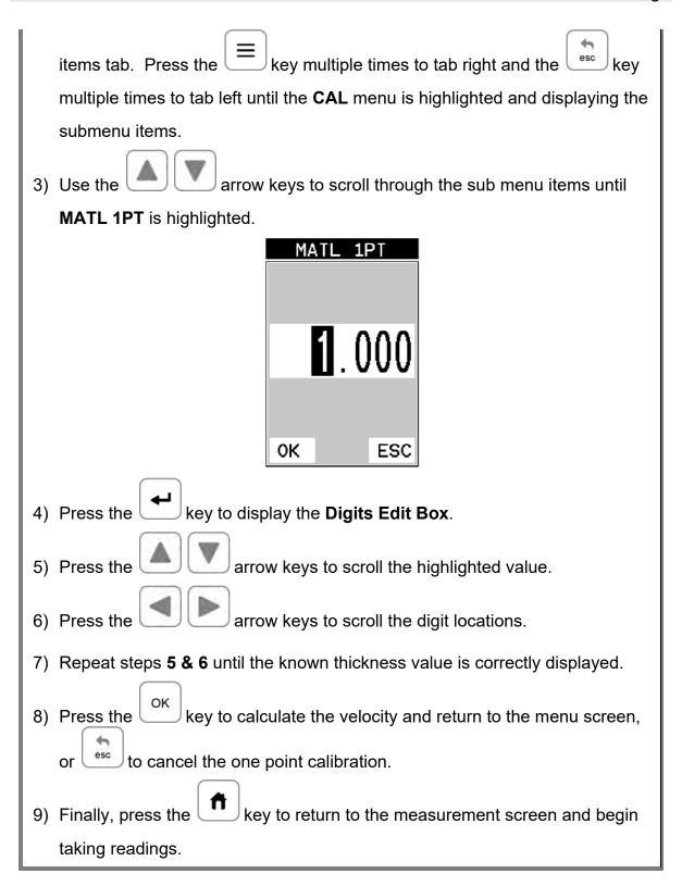
**Note:** CHECK YOUR CALIBRATION! Place the transducer back on the calibration point. The thickness reading should now match the known thickness. If the thickness is not correct, repeat the steps above.
