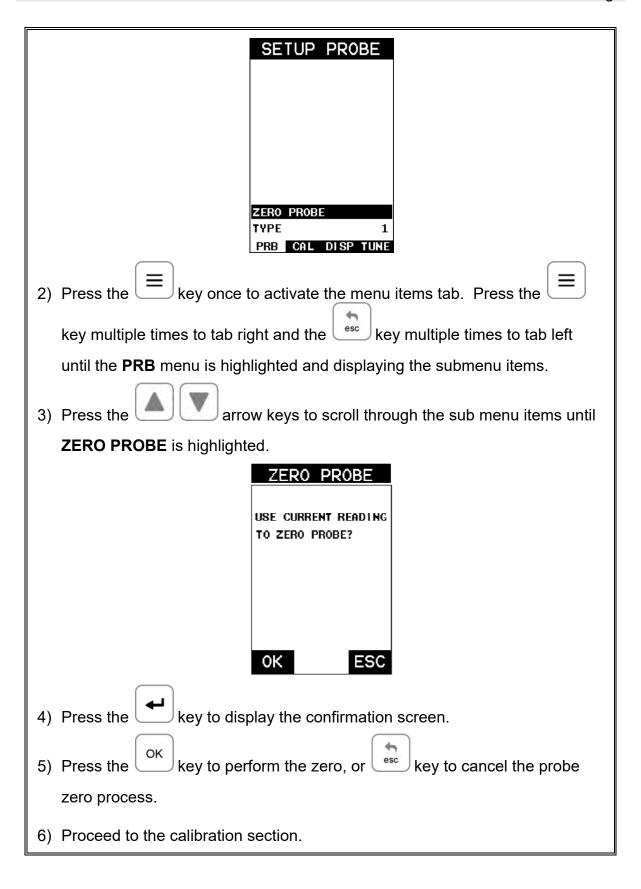
**Note:** The value that is displayed will change depending on the current velocity setting in the **MX2-DL**. Disregard the number that is displayed. **It is not important**. What is important is accurately performing the steps outlined above to insure reliability of the probe zero calculation.
