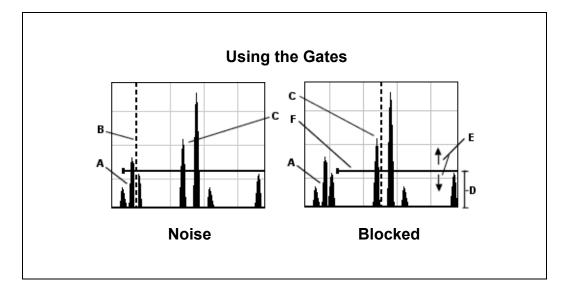
A = Surface noise or transducer ring. D = Threshold level
