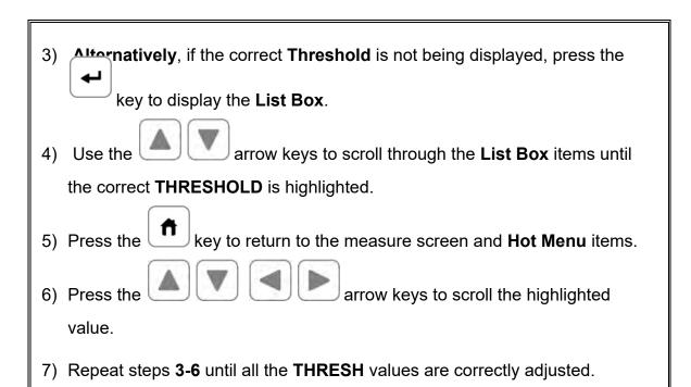
The user can also access and adjust the **Threshold** from the tabbed menus. However, this method is more tedious than making the adjustments using **the Hot Menus**. The procedure for using the tabbed menus is outlined below:
