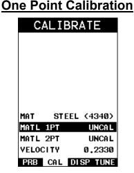
**Note:** Be sure that the probe zero has been performed prior to performing this procedure.
