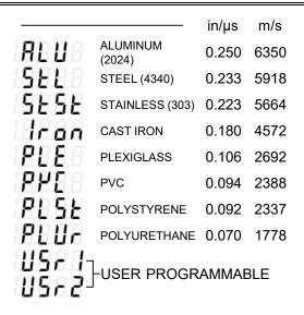
3) When the desired **MATL** setting is displayed, press the key to set the material velocity and return to the measurement screen.
