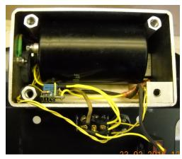
The Control Panel should only be removed by qualified personnel. When reinstalling the Control Panel to the Control Housing, extra care must be taken to manage the wiring harness, so individual wires are not pinched (or shorted) between the Panel and Housing.
