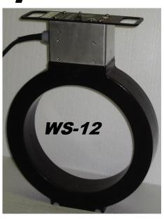
WS-Series Coils provide a powerful DC Pulse, once per second from a our CD (Capacitive Discharge) Power Supply. While the WS-Series uses a similar Coil Housings to Our WA and WP-Series Coils, it is slightly taller, built with a top panel with convenient handles. WS-Series Coils are completely different due to the unique CD Spike Power Supply for a field that extends into box end threads.
