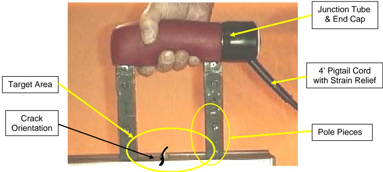
1. **Power Supply** – The WC-6UW is supplied power from the end-user’s 115VAC (or 230VAC) Grounded Power Supply or a 3VDC (or 6 VDC) Power Supply. The amperage draw for either power source is outlined at the end of this manual. No matter the type of electrical power supplied, full cautionary measures should be employed such as complete grounding and the use of a GFCI (Ground Fault Circuit Interrupter).
