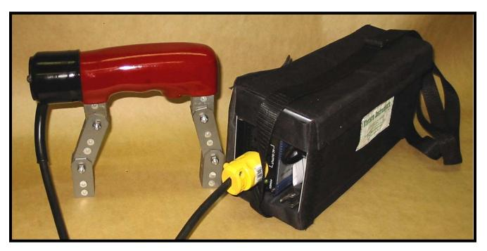
The W-PPS supplies AC Power to operate Western Instruments Yokes in an area where Mains Power is unavailable. The W-PPS is available in either 115VAC/60Hz or 230VAC/50Hz (W-PPSK) models. This Portable Power Supply weights 6kg / 13 pounds, so it is easily slung over the inspector's shoulder.
