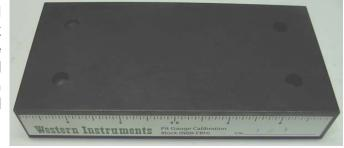
certification is only required if there is physical damage that may inhibit the use or accuracy of the Standard. As illustrated, the 4 Flat Bottom Holes are positioned in each corner of the sample, 19mm (0.75)") from each corresponding edge. N88-FBH's are supplied with a label, which includes a Centering Rule, for technician reference.
