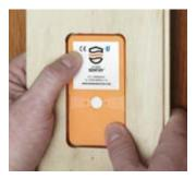
**IMPORTANT:** When installing the floor plank into the rest of the floor system, make sure that no adhesives or other constructionrelated materials interfere with the underside of the Floor Sentry. Keep in mind that each side (both top and bottom) of the Floor Sentry contains a sensor. Be sure to note and record the location of the Floor Sentry installation for future reference.
