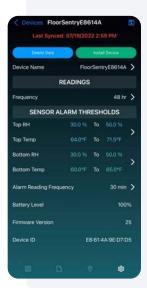
**NOTE:** For sensors, the alarm threshold defaults are 30–50% RH and 60–80 degrees F.
