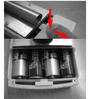
If the battery symbol appears in the measuring window resp. if a critical charge of battery is shown in the status, the batteries have to be changed IMMEDIATELY. If you do not use your humimeter device for a longer period, remove the batteries. For eventual resulting damages we cannot provide any warranty.
