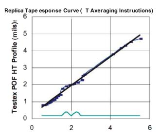
Laboratory-Determined Profile (Rt) Blue Curve = Replica Tape Profile Black Line = Straight Line Fit Green Curve (at bottom) = Measurement Uncertainty = Standard Deviation
