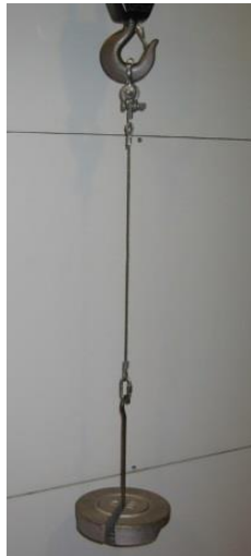
Figure 8: Free-hanging weight simulating material tension.
