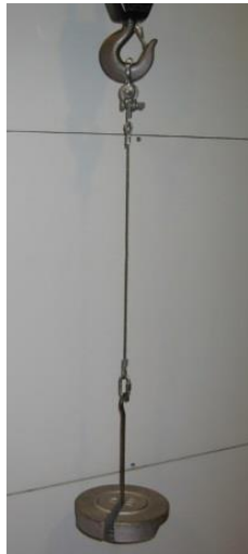
Figure 8: Free Hanging Weight simulating cable tension.
