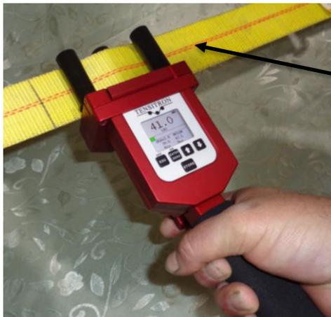
Note the routing of the band (under the outer guide rollers and over the center sensor roller) and the tension reading on the display.
