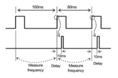
If the period of the external input is less than the setting of the delay time, the delay time is ignored and the ST-320BL flashes as if the delayed time equals 0.
