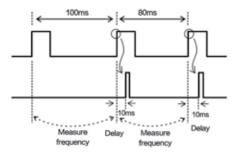
If the current period of external trigger input changes, the time of the flash is not accurate, because the time is calculated based on the previous measurement period.
